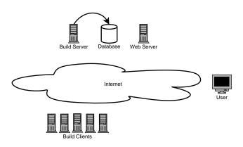
The *Build Server* feeds the log files to database, which allows asynchronous access.
