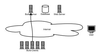
During the build the *Build Clients* writes a set of log files in a certain format. After the build is finished the *Build Clients* open again an ssh connection to the *Build Server* and pipe an archive including the log files to the server.
