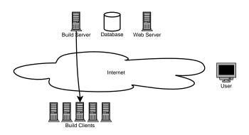
The *Build Server* opens a secure connection to the *Build Clients* via ssh and public key authentication. The server send a configuration for a single run, including which tests to run, etc.
