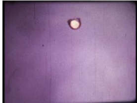
Molten oxide droplet surrounded by a vapor film
